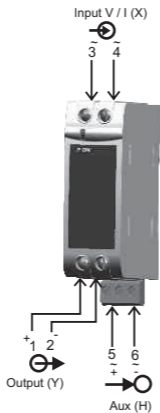
Fig. 6. Front View of Device for electrical Connections
